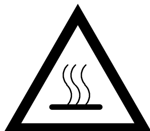
Fig. 25 Hot surface warning sign
