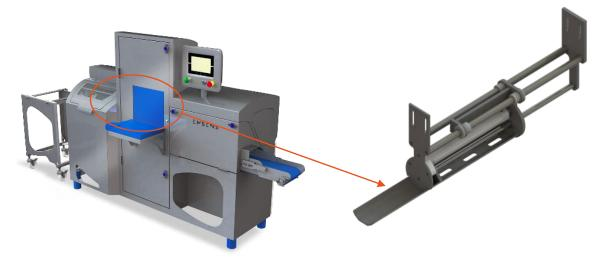
The product is positioned onto the exit belt and taken towards the exit of the machine.
